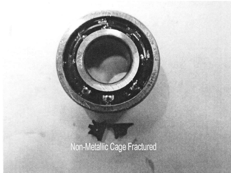
Figure 9. Duplex Thrust Bearing Distress
