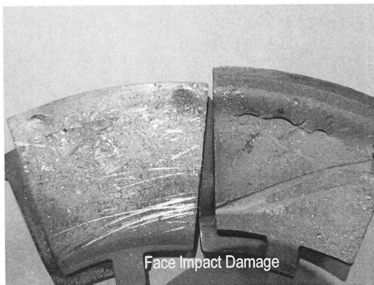
Figure 3. Seal Segment Damage
