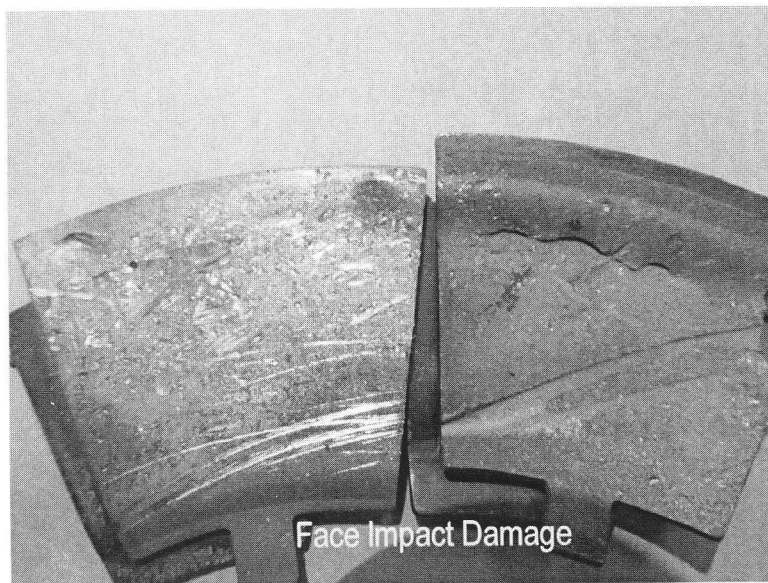
Figure 3. Seal Segment Damage
