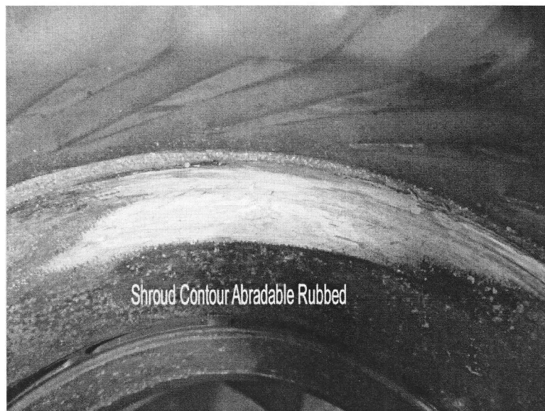
Figure 5. Air Inlet Housing Damage
