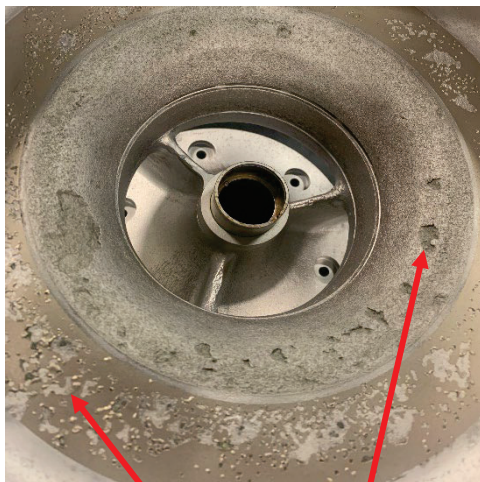
ABRADABLE MATERIAL DETERIORATED
