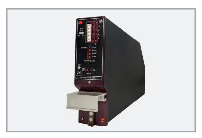
The L-3 Avionics PS-835 is a fully-enclosed power supply that provides continuous standby power for self-contained gyro horizons and essential flight instruments. The PS-835 Emergency Power supply is designed as a 24 VDC (nominal) emergency power source for prolonging the operation of a connected standby attitude indicator when the aircraft's main power bus has de-energized. The is designed to easily fit into the existing avionics shelf.
