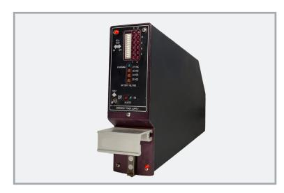
The L-3 Avionics PS-835 is a fully-enclosed power supply that provides continuous standby power for self-contained gyro horizons and essential flight instruments. The PS-835 Emergency Power supply is designed as a 24 VDC (nominal) emergency power source for prolonging the operation of a connected standby attitude indicator when the aircraft's main power bus has de-energized. The power supply unit is designed to easily fit into the existing avionics shelf.
