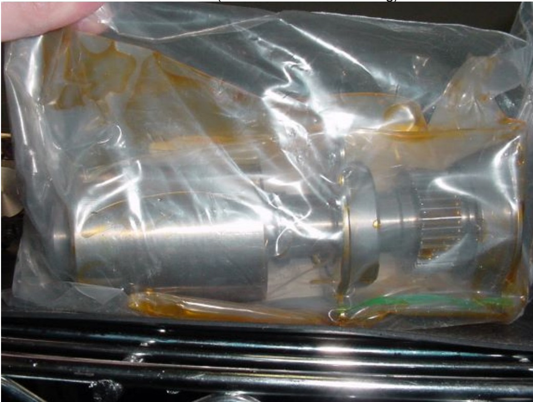
BSG pinion (magnet migrated forward)
