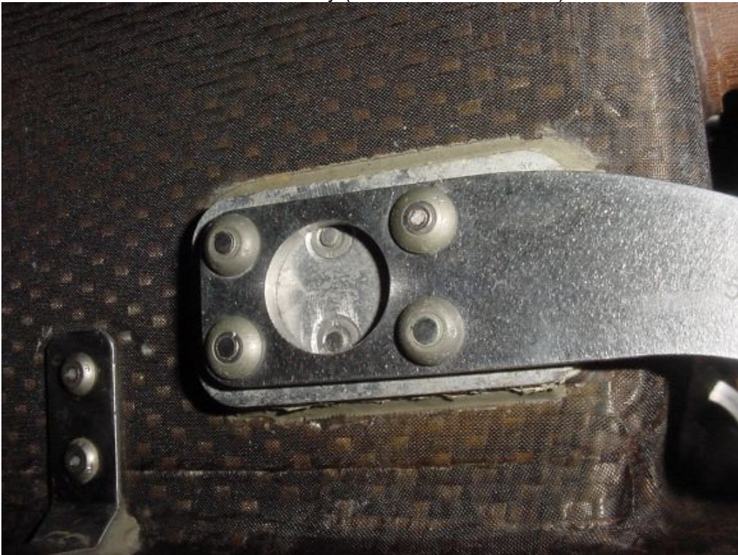
Air intake plenum (corrosion at shims)
