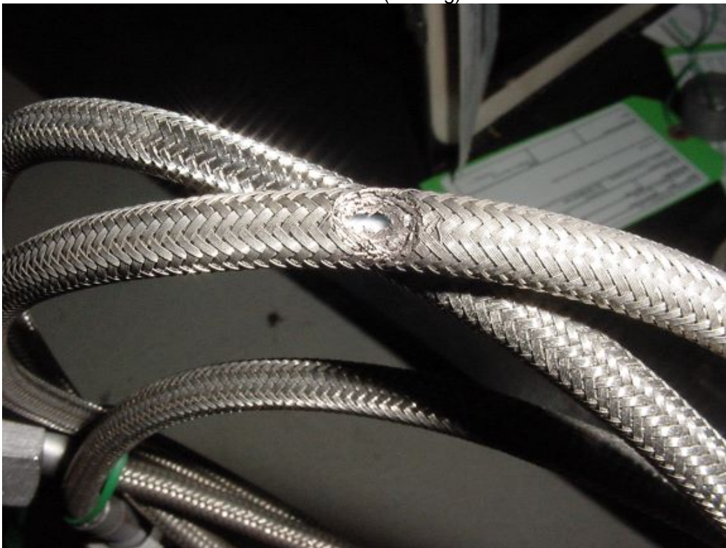
Igniter cable (chaffed through)
