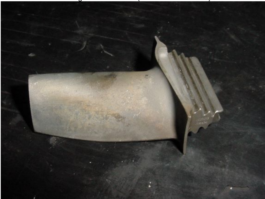
2 ND stage turbine blades (cracks in fir trees)
