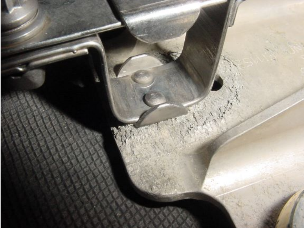
Bracket assembly (corrosion delamination)
