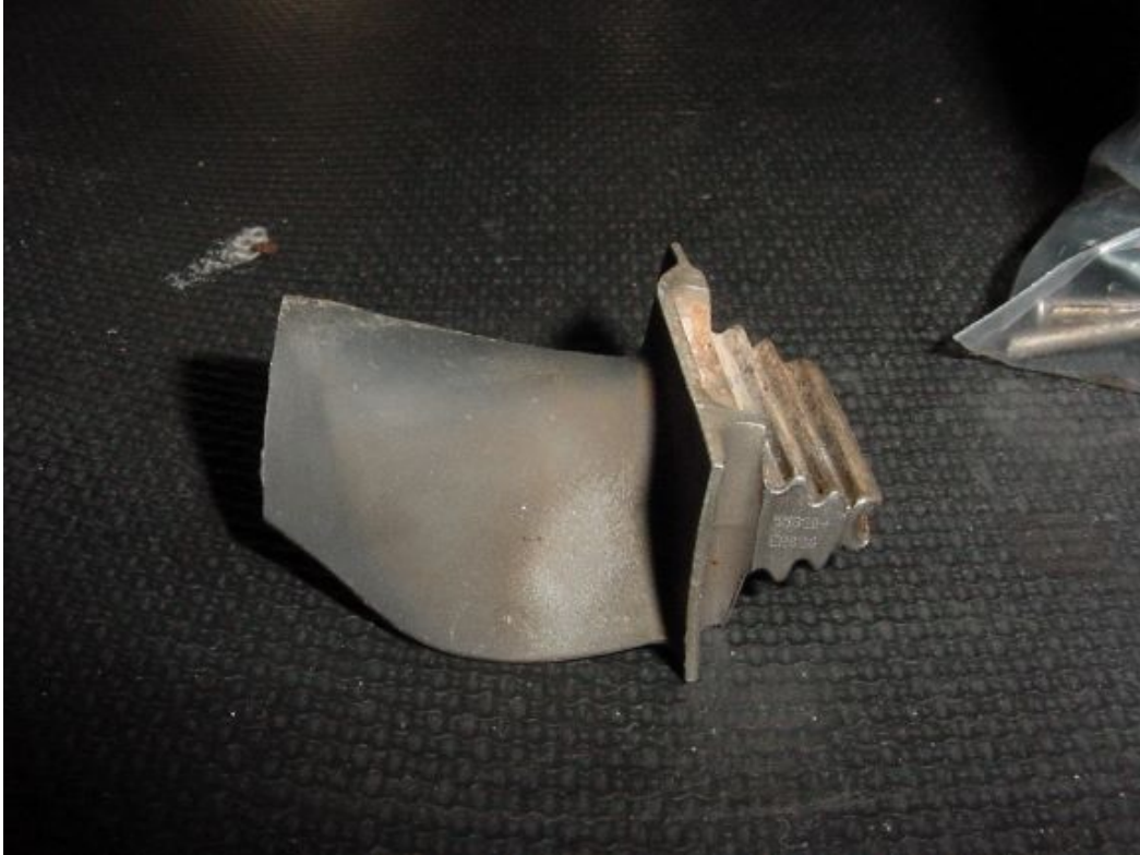
1 ST stage turbine blades (cracks in the fir trees)
