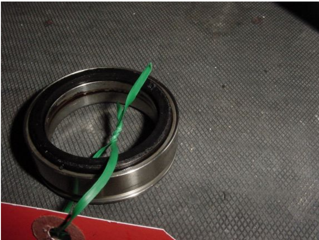
Carbon seal (carbon chipped/pitted)
