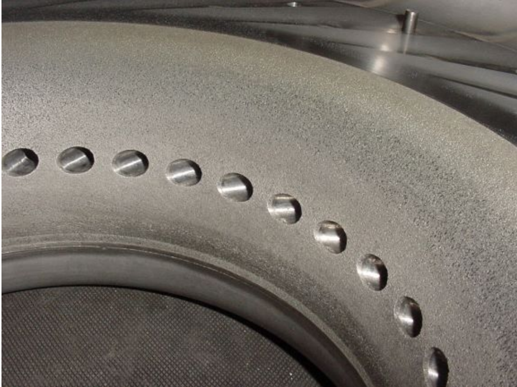
Compressor shroud (abradable eroded)
