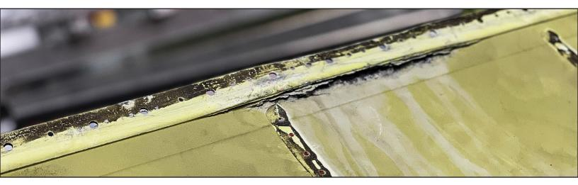
One of the most common issues on the Hawker 800 Series is skin corrosion on the leading edges. Skin corrosion may not be visible initially, which could make ie difficult to identify.
